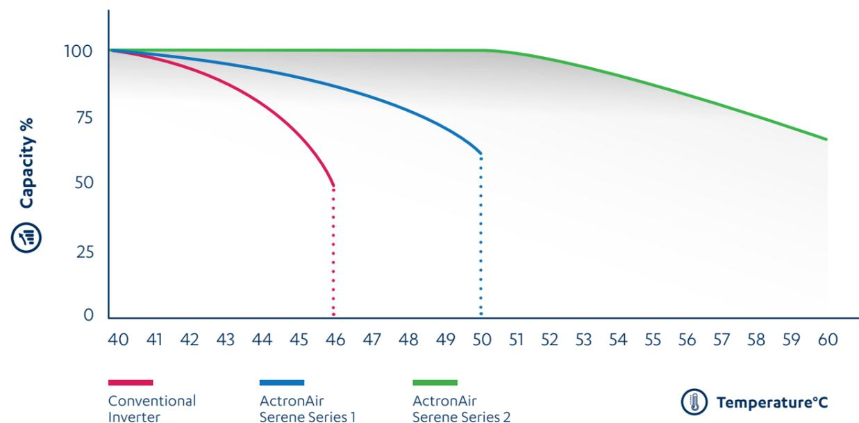
\*Based on the 2.6kw Serene 2 system. Outside air temp of 50.01 °C, indoor temperature of 32.01 DB / 23WB
