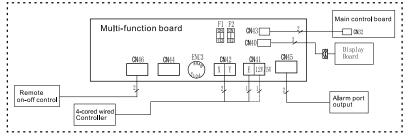
When connecting to 4-core wired controller:
