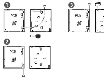
4. Notch the part for the wiring to pass through with a nipper tool.
