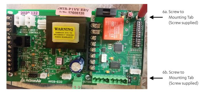
Step 6. Use the supplied screws to secure the BMS Board to the mounting tabs
