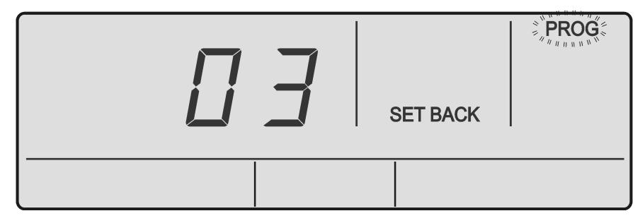
3. Press the **PROG** button to enter Program Menu 03. Display will show Set back display **ON** field is blinking.
