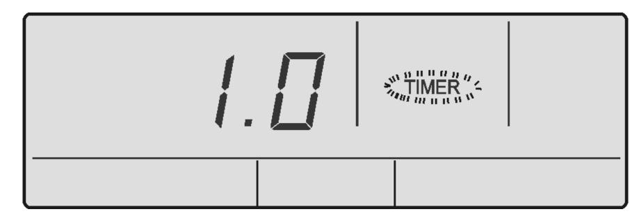
3. 3 seconds after the last press of the ^ or buttons or simply press **TIMER**, the display will go back to the main screen and the ON Timer countdown will start. The unit will turn On after the timer has expired.
