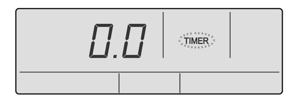
2. Press the ^ ① or ~ buttons to select the desired time for the system to remain operating before turning Off. The maximum adjustable timer hours are 24 with 0.5 hour (30 minute) adjustable increments.
