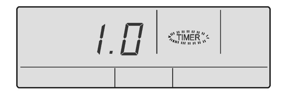
3. 3 seconds after the last press of the or buttons or simply press TIMER, the display will go back to the main screen and the OFF Timer countdown will start. The unit will turn Off after the timer has expired.
