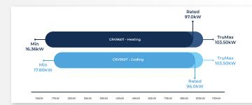
When the temperature outside soars or plummets. TruMax functionality allows the system to continue performing at higher capacities, meaning it can be counted on to provide powerful cooling or heating when it's needed the most.
