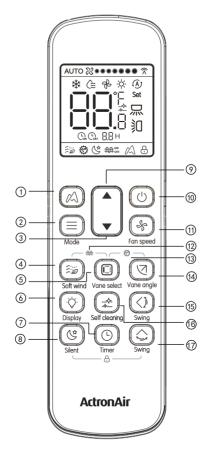
Figure 3.1 External view of remote controller
