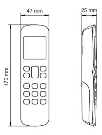
Figure 2.1 Dimensions of remote controller
