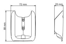
Figure 2.2 Dimensions of remote controller bracket
