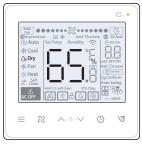
In dry mode, press "  $\wedge$  " and "  $\vee$  " to change humidity in the range of 35-75%.
