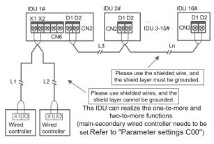
The one-to-more function must be set for the wired controller.(Refer to "Parameter settings N37") After the communication between the wired controller and IDU lasts 3 minutes and 30 seconds, the control can be implemented.
