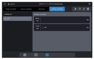
Note: As you may have noticed, the system does not determine the date for the execution of the holiday template. The holiday template is created by following the above steps, but it is not used. The template needs to be used in the schedule. The system will specify the date on which the template is executed only if the holiday template is used.
