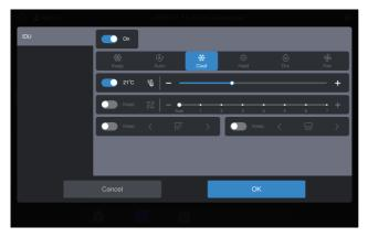
Note: When IDUs support single parameter control, you may not select other parameters. The actual operating parameters of the IDUs depend on the logic of the IDUs, which are generally those of the last operation of the IDUs.
