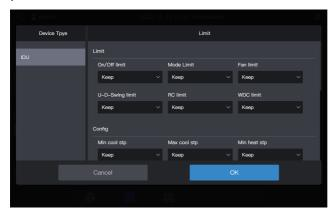
Note: The locking parameters displayed on the interface may exceed the actual lockable parameters of the IDU. When this parameter is selected, the actual IDU does not operate.
