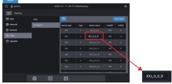
Mode 2: Modify the device name on the "Device monitoring" interface.
