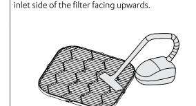
Clean the filter with a vacuum cleaner, with the air
