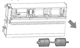
(5) Loosen the fastening screws for the wind wheel and remove the coupling and motor shaft.
