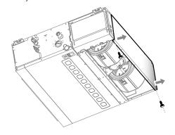
2 Rotate the portion of the top cover that covers the propeller housing by approximately 30 degrees around the long U-shaped hole, as shown in the figure.
