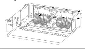
(5) Move the upper propeller housing 50mm backward.
