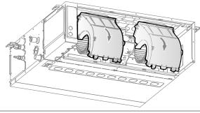
(7) Remove the lower propeller housing in a backward direction.
