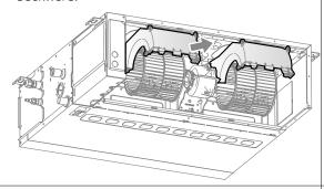
(6) Make the propeller housing rotate more than 90° downward along the wind wheel.
