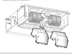
(8) Note: Installation notes are as follows: The slot and latch bolt, and the limiting groove and side wall edge should be aligned first, and then be fastened; Check whether the limiting groove, positioning rod and buckle are installed in place, and the limiting latch bolt shall enclose the outside of the propeller housing.
