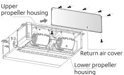
Remove the two screws from the top cover and rotate the portion of the top cover that covers the propeller housing by approximately 30 degrees around the long U-shaped hole, as shown in the figure.
