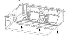
3 Remove the lower propeller housing in a downward diagonal direction.
