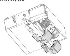
4 Loosen the fastening screws for the motor sealing plate and wind wheel.
