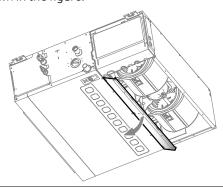
③ Press the buckle of the upper propeller housing, and rotate the lower propeller housing around the front edge of the lower propeller housing by about 30 degrees.
