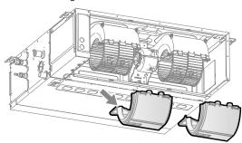
4 Loosen the screws on the upper propeller housing.
