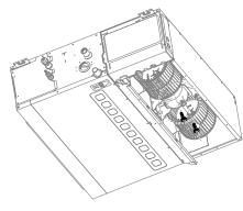
(5) Remove the motor and wind wheel together.
