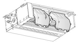
Slanting downward, remove the lower propeller housing.
