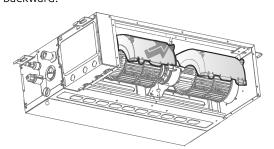
(6) Make the propeller housing rotate more than 90° downward along the wind wheel.
