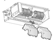
8 Loosen the fastening screws for the motor sealing plate.
