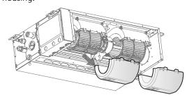
4 Loosen the screws on the upper propeller housing.
