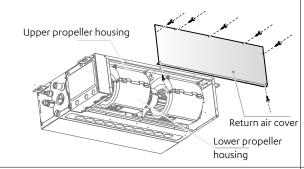
Press the buckle of the upper propeller housing, and rotate the lower propeller housing around the front edge of the lower propeller housing by about 30 degrees.
