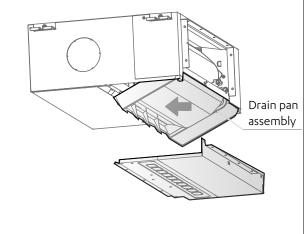
Shift the drain pan downwards until the drain pan is removed from the unit body
