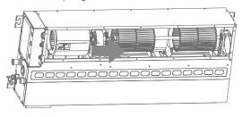
Remove the wind wheel, connecting shaft and coupling together.
