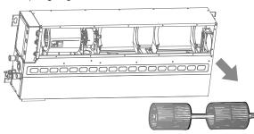
5 Loosen the fastening screws for the wind wheel and remove the coupling and motor shaft.
