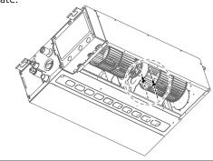
Remove the motor and wind wheel together; unscrew the screws securing the wind wheel in place and remove the wind wheel and motor.
