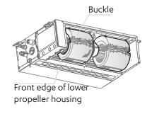
Slanting downward, remove the lower propeller housing.
