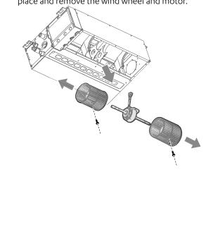
(II) Note: Installation notes are as follows: The slot and latch bolt, and the limiting groove and side wall edge should be aligned first, and then be fastened; Check whether the limiting groove, positioning rod and buckle are installed in place, and the limiting latch bolt shall enclose the outside of the propeller housing.
