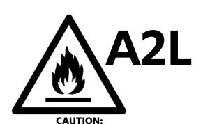
The system is charged with flammable refrigerant, safety checks are necessary to ensure that the risk of ignition is minimised.
