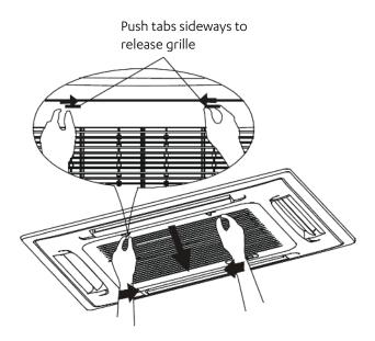
Step 2. Remove the filter from the grille.
