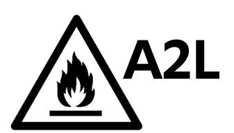
The system is charged with flammable refrigerant, safety checks are necessary to ensure that the risk of ignition is minimised.
