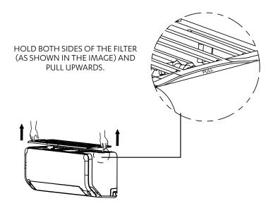
Filter is held in place by mag pull magnets, which helps in easily re-fitting the filter after cleaning.
